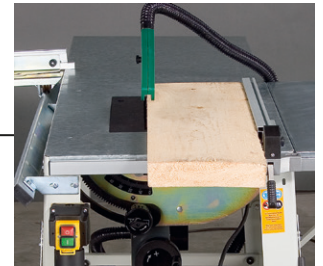
The rip fence is designed for peeling boards, rip cutting, bevelling, and angled cutting
