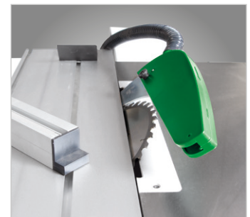
The saw blade pivots through 45°.
