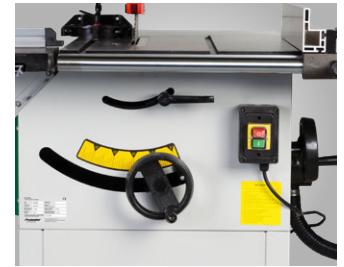
Features precise, easy-action height and angle adjustment of the sawing unit thanks to easy to use handwheel.
