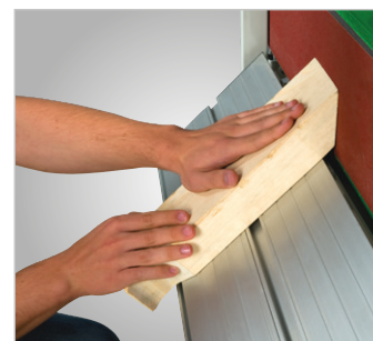
Mitres up to 45° by pivoting the longitudinal table
