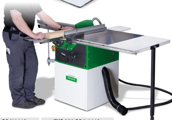
The cross cut stop supports mitre cuts on both sides, 45°
