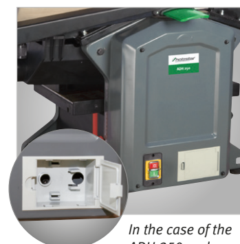
ADH 305 Features an integrated storage compartment
