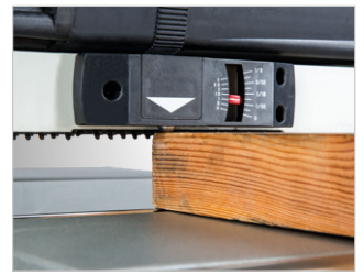
Mechanical material removal display
