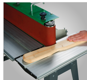
Easiest possible approach to sanding radii
