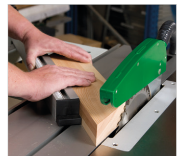
The cross cut stop supports mitre cuts on both sides, 45°
