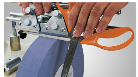
Jig for scissors/shears (Art. no.: 5760058)
