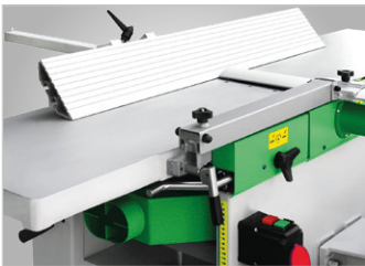
Large grey cast iron thickening table with polished surface
